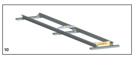
Finally, you can confirm the sideways level of the rails by using a spirit level.
