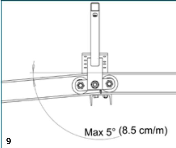
On models with two carriage axles, joints can be placed at an angle according to picture 9.
