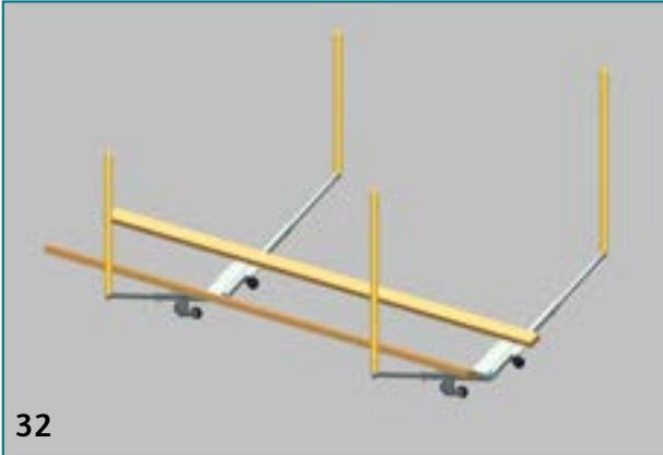
In VR-1500 model POM tandem wheels are installed to both carriage axles.
