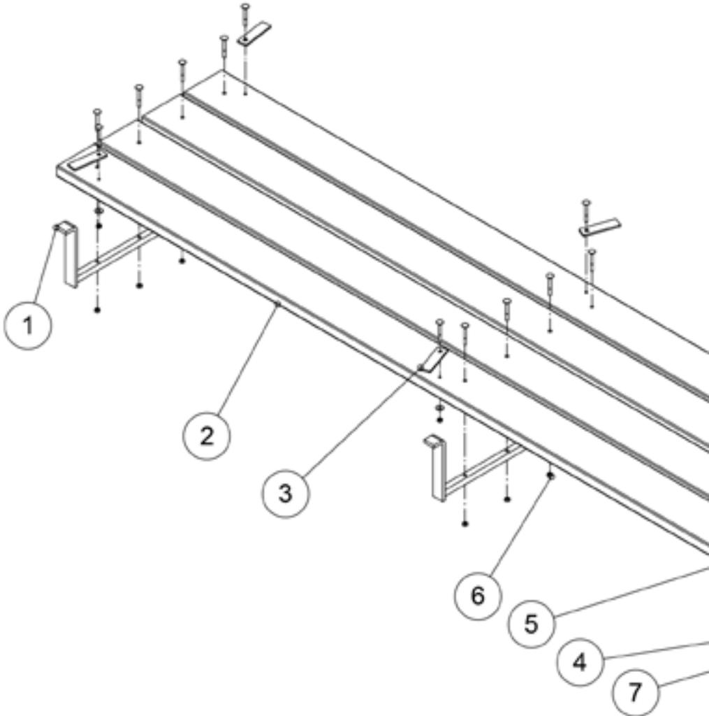
Drill three 8 mm holes in the edge planks of the walking platform for the installation of the locking plates (part 3). Drill the holes on the same side at a distance of 30 mm from the outer edge of the planks and at a distance of 100 mm from the ends of the planks. Drill the holes of the middle locking boards at a distance of 50 mm from the middle frame bar.
