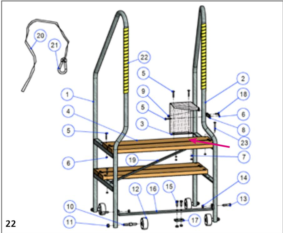
Attach the step boards lightly and put the wheels in place. The uppermost step board can be attached to the front or rear part of the stairs (see arrow) with consideration to the shape of the boat's bow.
