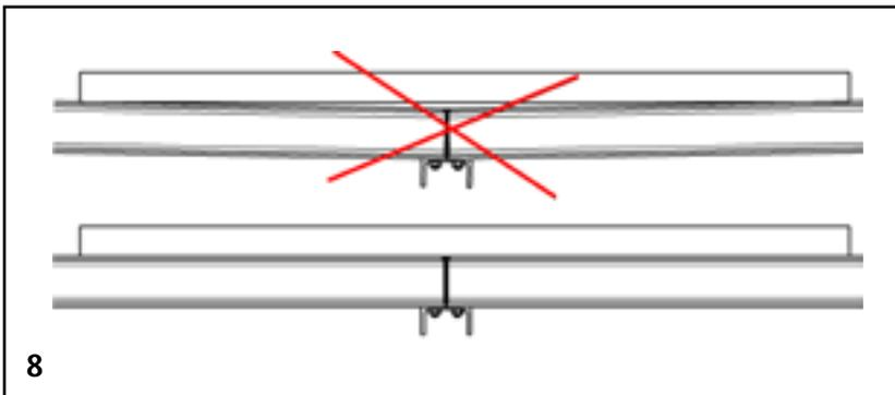
The rails should be assembled as straight as possible at the assembly stage with e.g. a guide rail. Avoid joints that sink down in particular. The straightness of the rail line is especially essential on models with three carriage axles (VR-2000, VR-2500).
