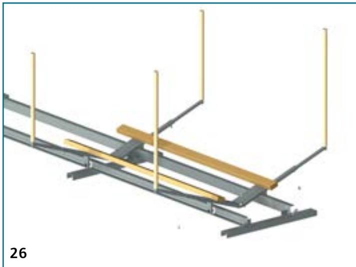
Adjust the width of the side guides according to the width of the boat and tighten the screws.
