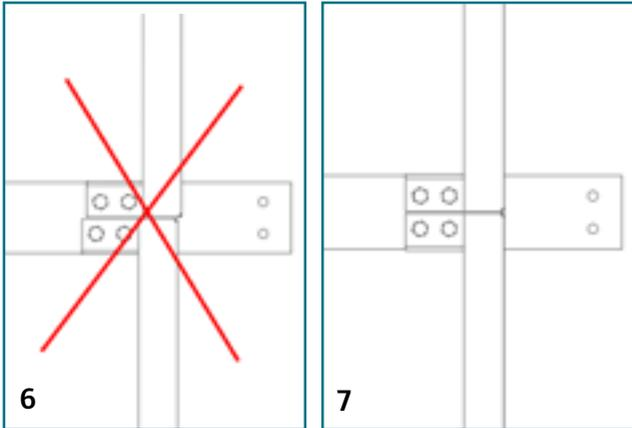
To prevent the wheels of the carriage from getting stuck at the joints of the beams, install the beams without any staggering (drawings 6 and 7).
