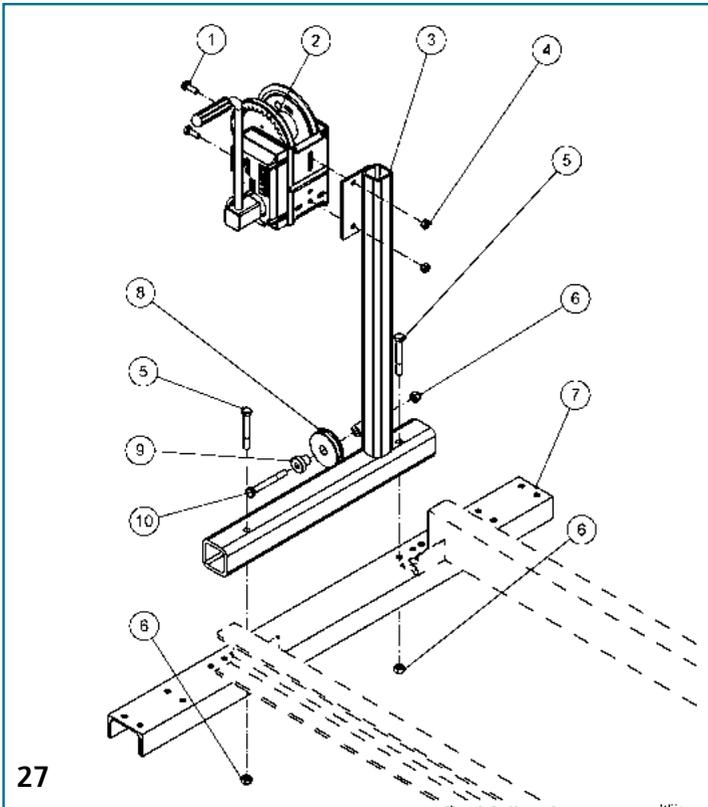
Attach the mounting beam of the winch (part 3) to the horizontal beam of the top end (part 7) with two M12X90 hex screws (part 5) and two M12 nuts (part 6). Attach the spur (part 8) with the help of bushing (part 9) and the hex screw M12x100 (part 10) and lock them with the M12 nut (part 6).
