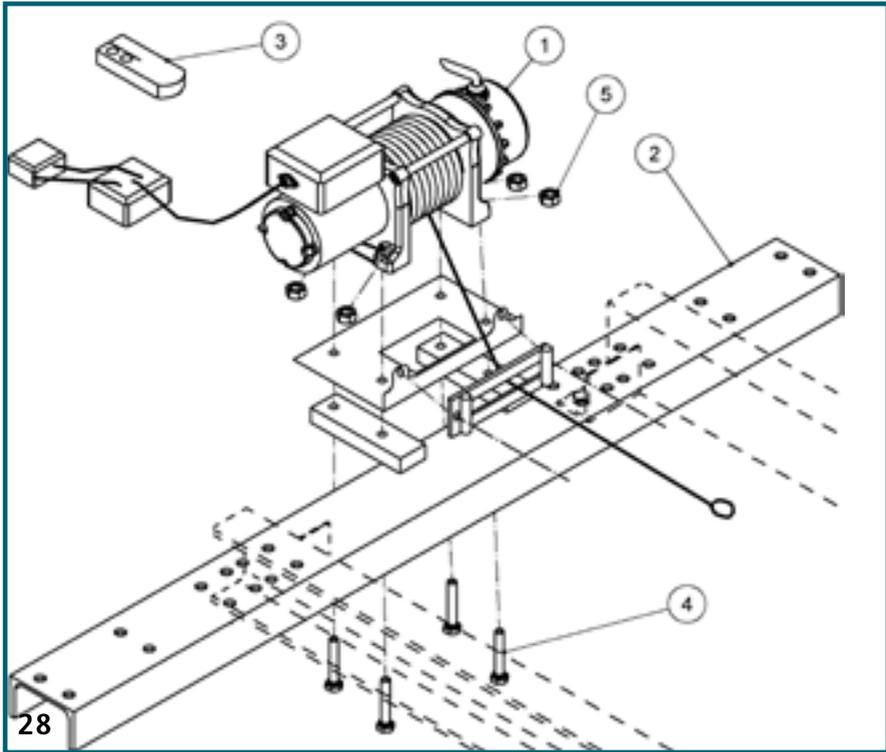
Install the mounting beam (part 2) of the electric winch (part 1) to the top end of the rails. Place the black mounting plate between the mounting beam and winch. After that, mount the fairlead to the mounting plate. Attach the winch to the mounting beam with four M8x45 screws and nuts (part 4) as shown in the picture. Part 3 is the winch's remote control.
