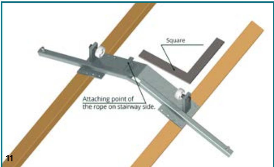
The planks of the carriage can be installed to the inner or outer holes according to the shape of the boat's hull, taking into account the raised boards etc., so that they are fixed at the same location on both sides. In most cases, the best place for the planks is at the outer holes. The planks are placed in the inner holes only if the boat or its hull is particularly narrow.
