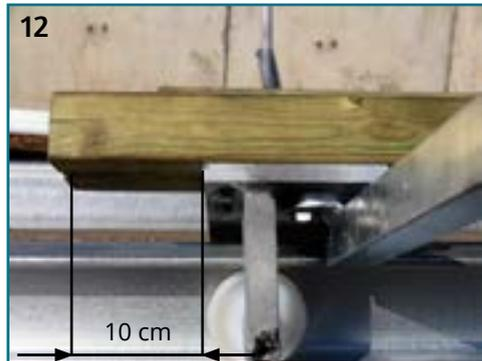
When the carriage has been assembled, push the carriage's v-bodies from the top of the rails in to place so that the wheels go in to the U-beams (picture 13). **Prevent the carriage from sliding into the water during the installation!**
