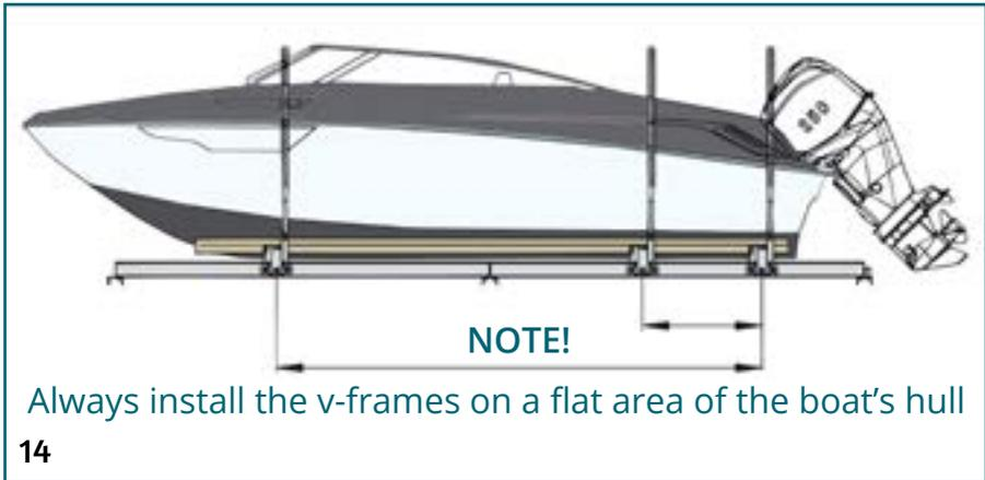
Install the v-frames according to the picture 14. The distance between the outermost v-bodies is within the flat area of the boat's hull. Place the middle v-body approx. 1/4 from the rearmost v-body to the front v-body.
